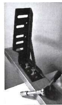
11A This option is for heavier or larger bed heads. Attach with self tapping screws and coach bolts. Before screwing in coach bolts pre-drill with a 3mm drill bit and then screw in with a spanner or socket and ratchet. Tighten firmly but don't over tighten.
