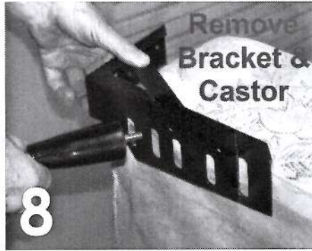
8 Remove castors and bed head brackets from the ensemble ready for attaching to bed head.
