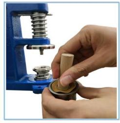
Whilst holding the top die, use the wood dowl to push the cap firmly into the base.
