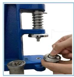
Lay back component of button facing down inside the bottom die.
