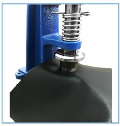
Place fabric on the nylon cutting block. Fold or stack material to cut more pieces at a time. Pull on handle to cut round button covers.
