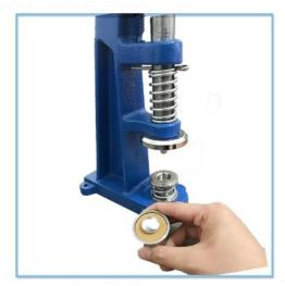
Turn the top die down and place a single round button cover and single button mold top in centre as shown in the picture.
